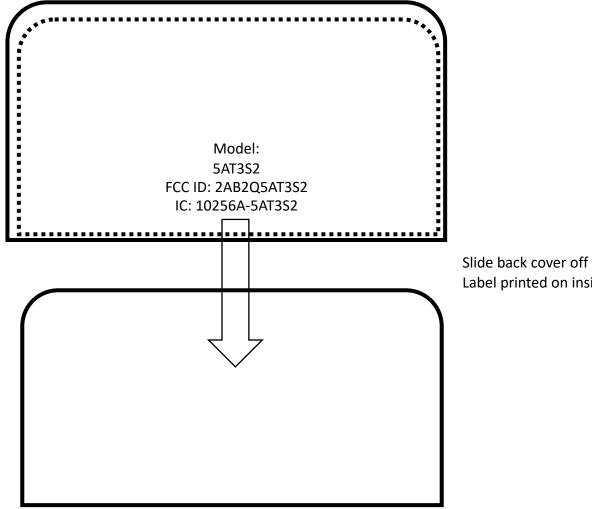
Slide back cover off the device. Label printed on inside of device.
