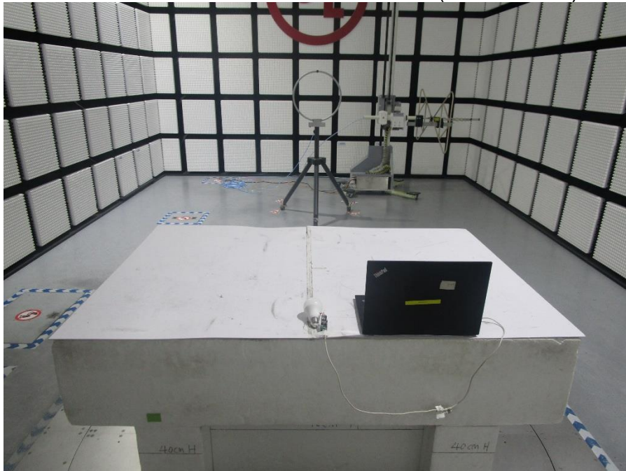
RADIATED RF MEASUREMENT SETUP (Below 30MHz)
