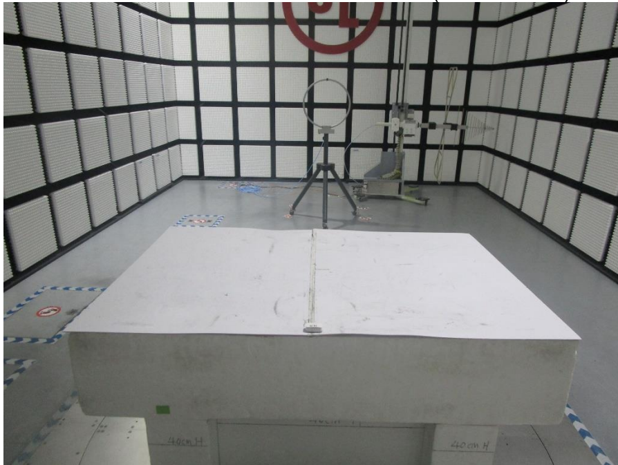
RADIATED RF MEASUREMENT SETUP (Below 30MHz)
