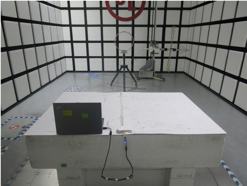
RADIATED RF MEASUREMENT SETUP (Below 30MHz)
