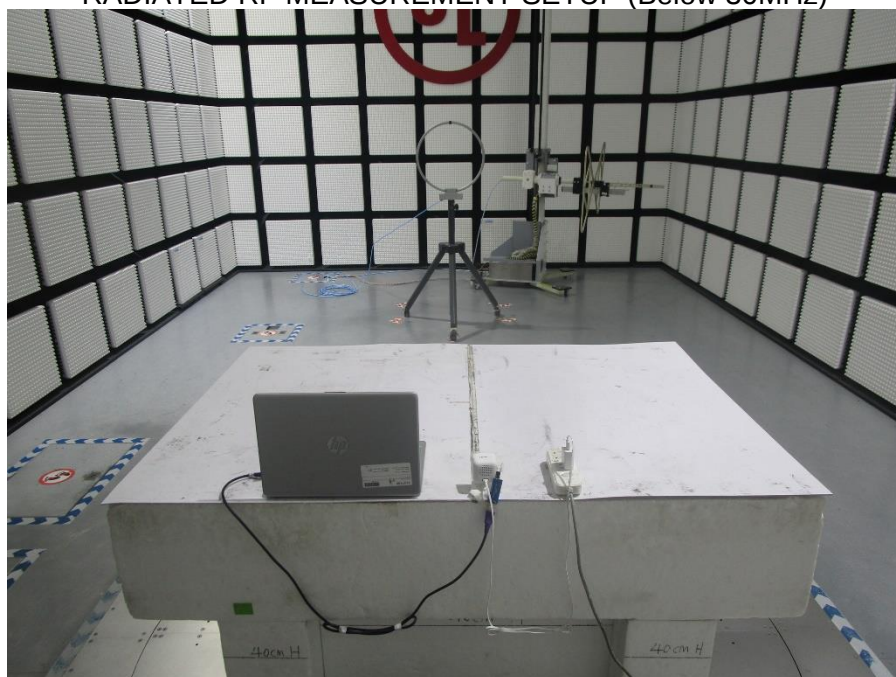
RADIATED RF MEASUREMENT SETUP (Below 30MHz)
