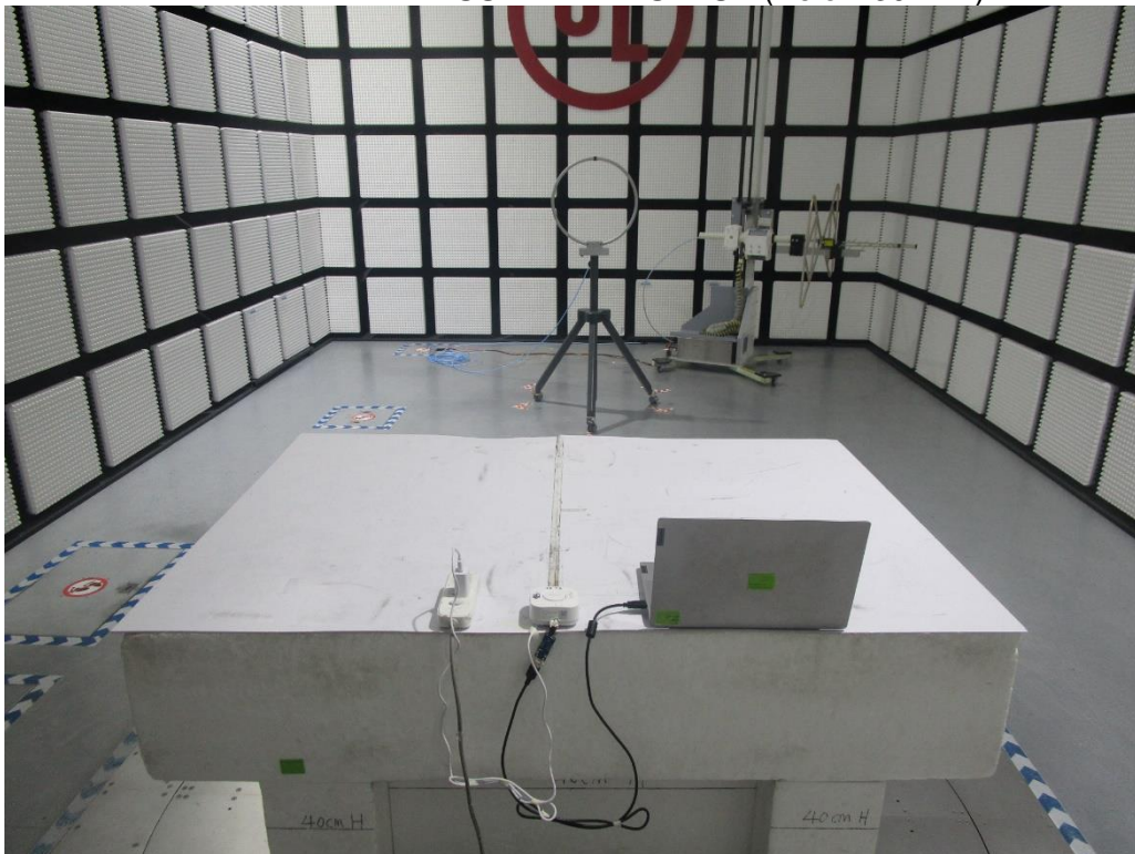
RADIATED RF MEASUREMENT SETUP (Below 30MHz)
