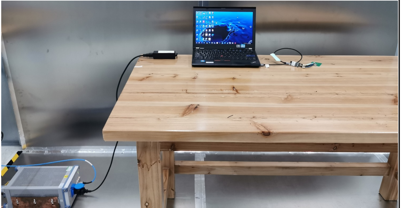
Photograph 3: Set-up for Conducted Emission on AC mains
