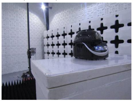
Conducted disturbance voltage at mains ports (150KHz-30MHz)
