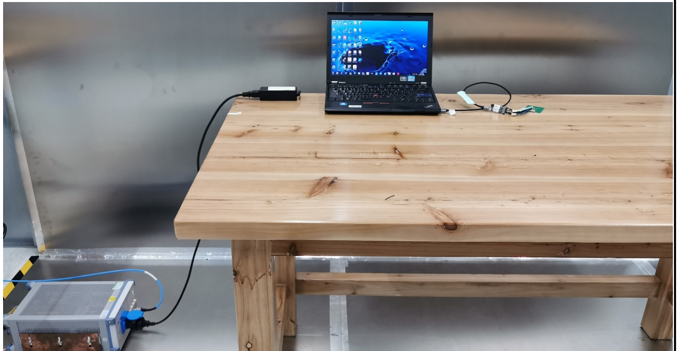
Photograph 3: Set-up for Conducted Emission on AC mains
