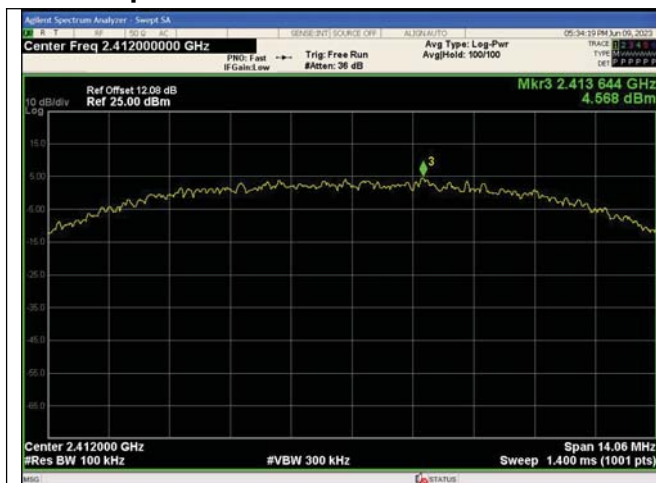
In-Band Reference Level IEEE 802.11b_Channel 1_20MHz_Antenna 0
