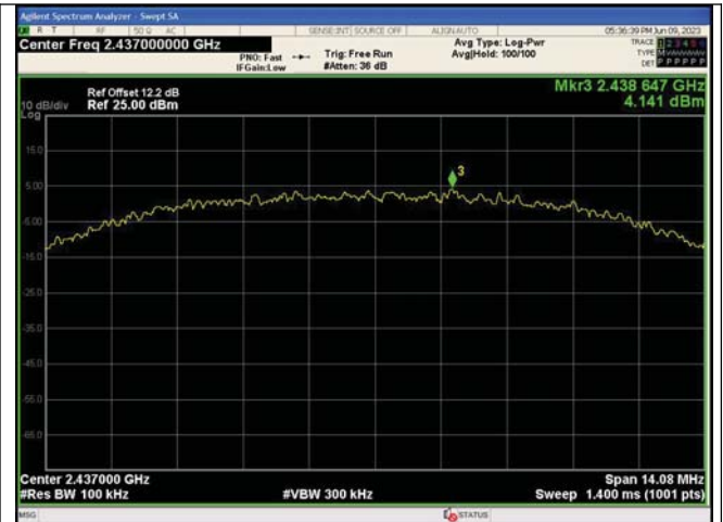
In-Band Reference Level IEEE 802.11b_Channel 6_20MHz_Antenna 0
