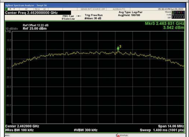
In-Band Reference Level IEEE 802.11b_Channel 11_20MHz_Antenna 0
