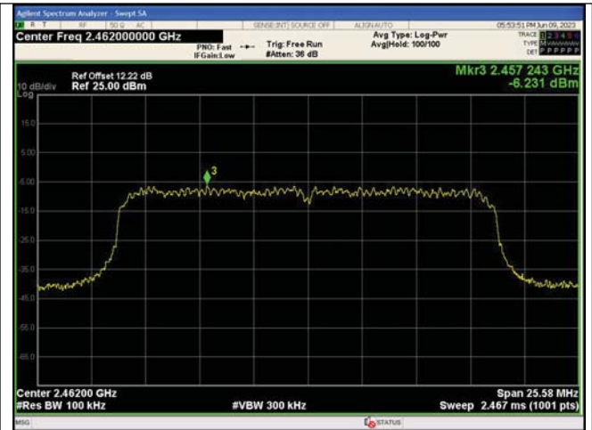
In-Band Reference Level IEEE 802.11n_Channel 11_20MHz_Antenna 0
