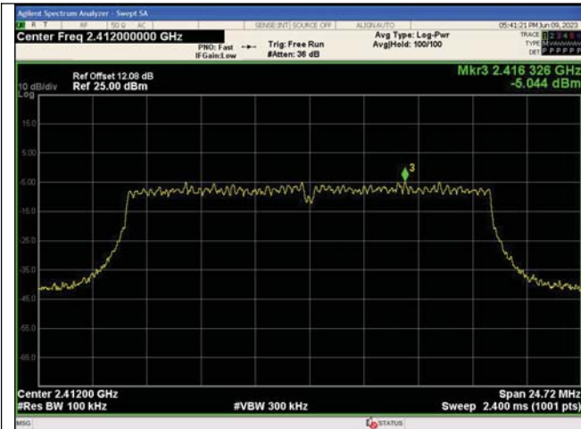
In-Band Reference Level IEEE 802.11g_Channel 1_20MHz_Antenna 0
