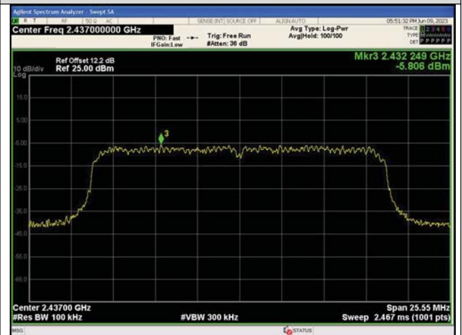
In-Band Reference Level IEEE 802.11n_Channel 6_20MHz_Antenna 0
