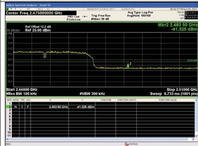
Out Of Band Emission IEEE 802.11n_Channel 9_40MHz_Antenna 0
