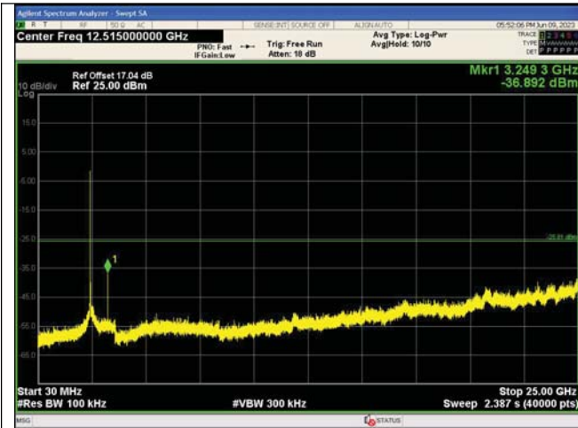
Spurious Emissions IEEE 802.11n_Channel 6_20MHz_Antenna 0
