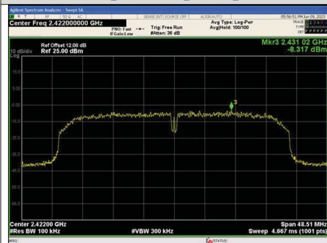
In-Band Reference Level IEEE 802.11n_Channel 3_40MHz_Antenna 0
