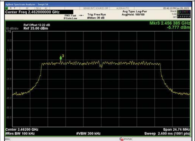
In-Band Reference Level IEEE 802.11g_Channel 11_20MHz_Antenna 0
