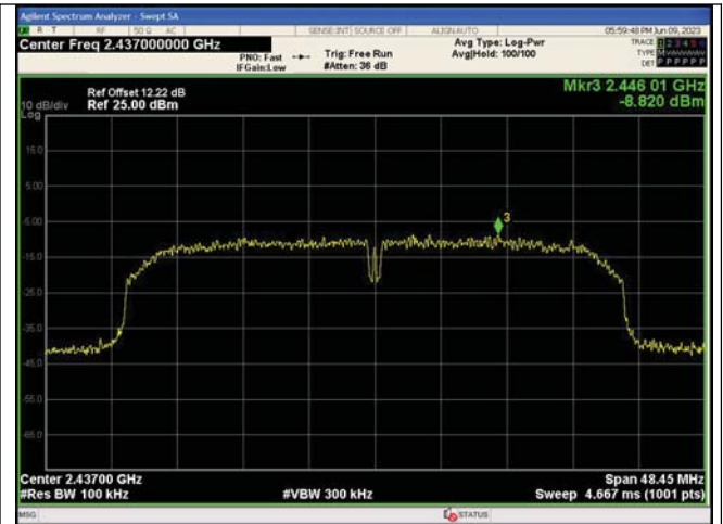
In-Band Reference Level IEEE 802.11n_Channel 6_40MHz_Antenna 0
