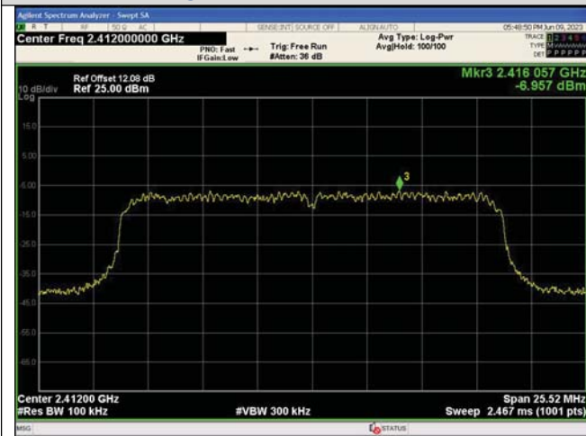
In-Band Reference Level IEEE 802.11n_Channel 1_20MHz_Antenna 0
