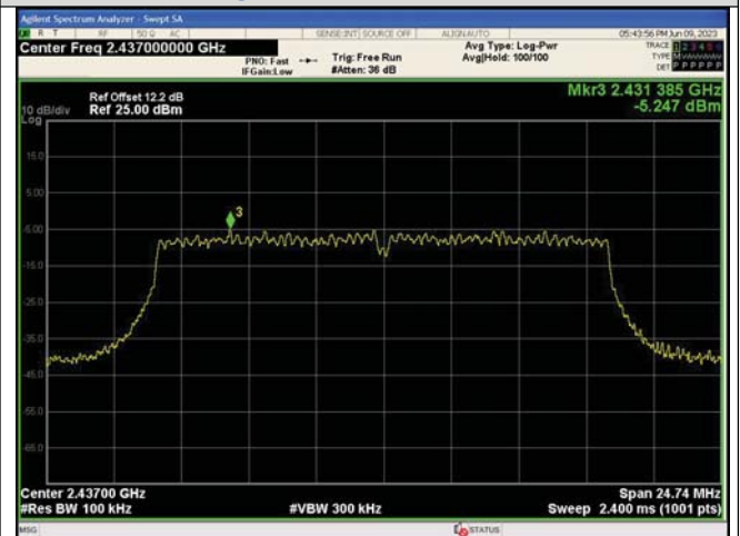
In-Band Reference Level IEEE 802.11g_Channel 6_20MHz_Antenna 0
