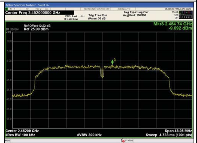
In-Band Reference Level IEEE 802.11n_Channel 9_40MHz_Antenna 0
