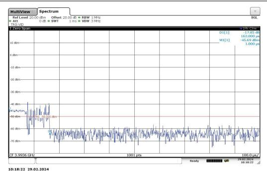
Test result for Slow update Mode: When the UWB is activated for indoor operation and the device is moving:
