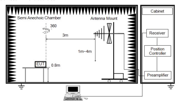
The setting of the spectrum analyzer:
