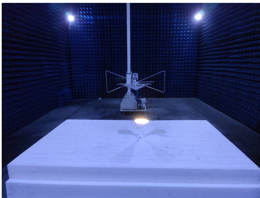
Photo of Radiated Emission Measurement (Below 1G)
