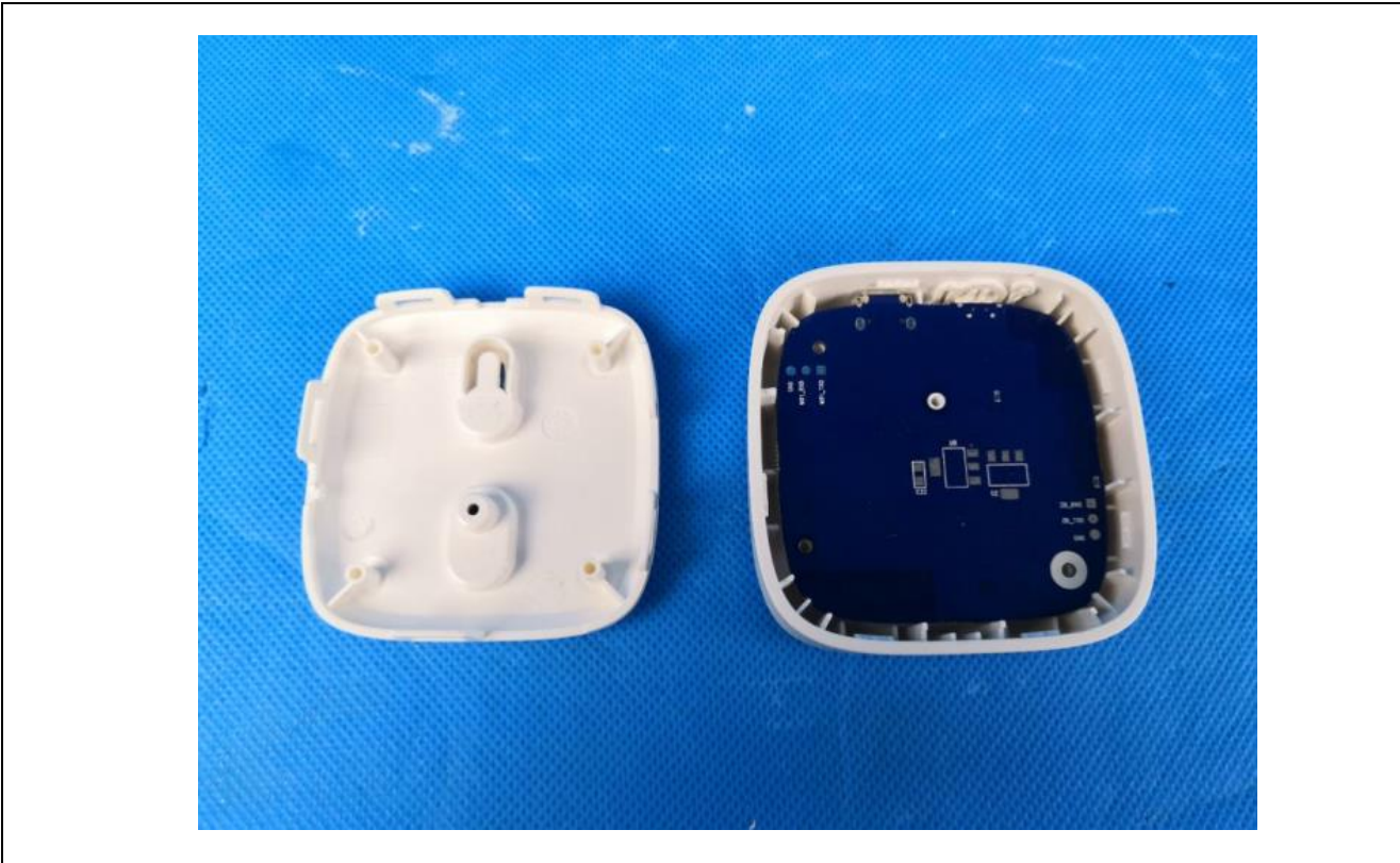
Details of: PCB component side view for model 7B-GW-ZWA-H0-01
