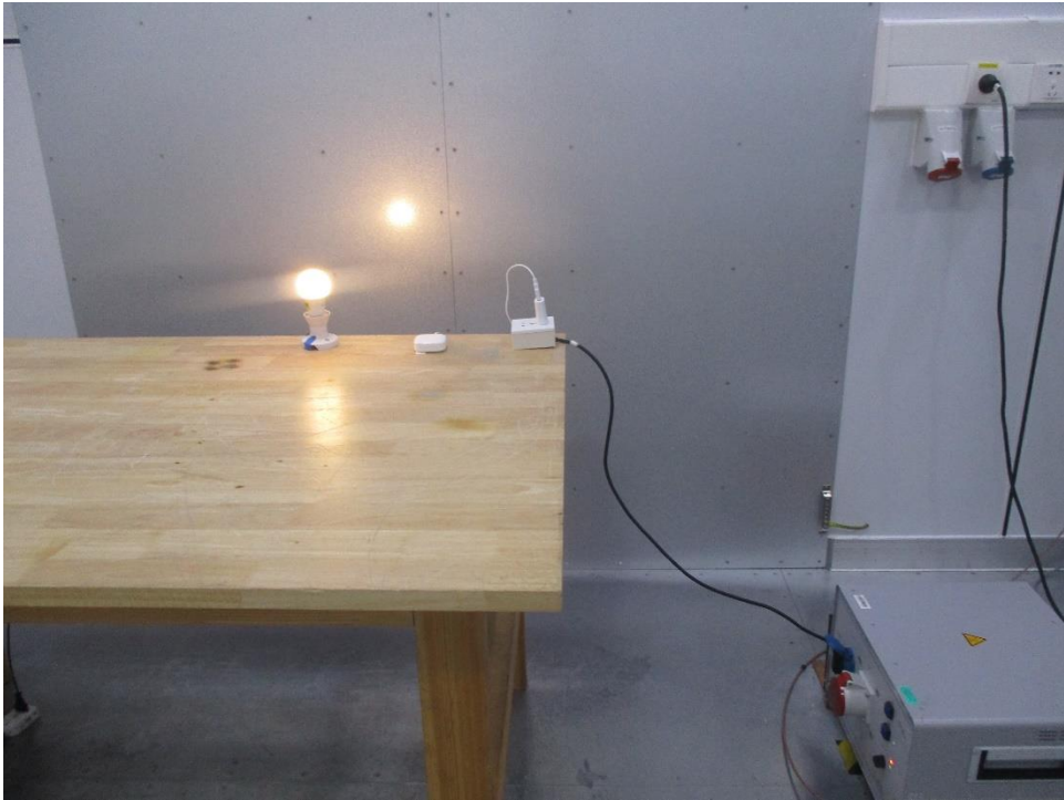
Conducted Emission test
