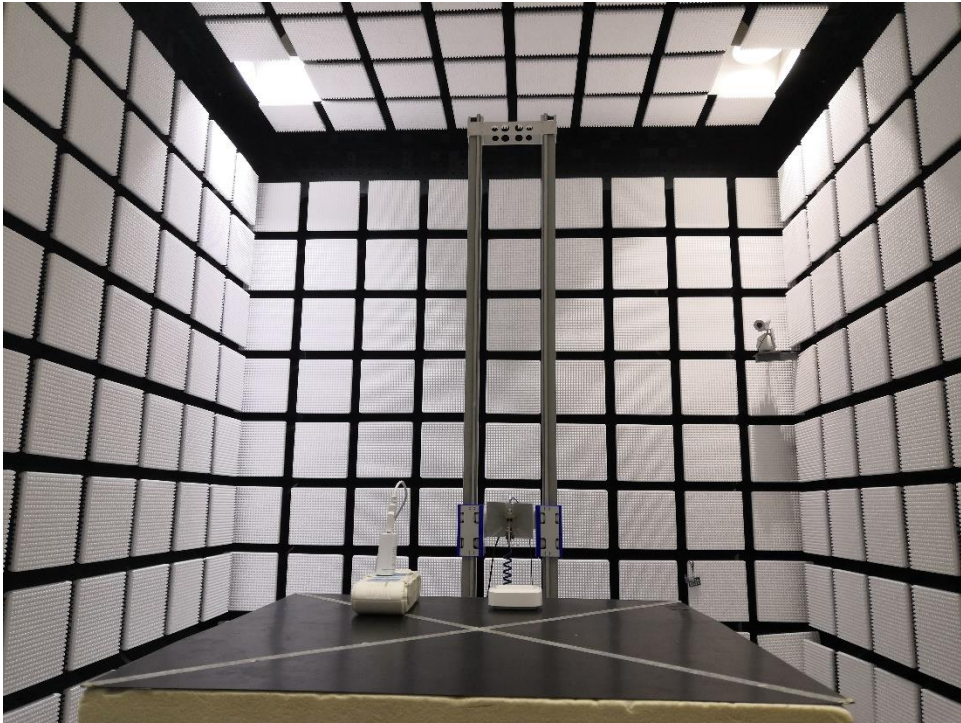
Radiated Emission test Above 1GHz
