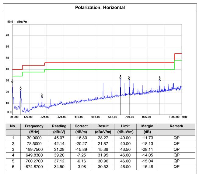
Result = Reading +Correct (Amplifier Factor + Cable Loss + Antenna Factor)
