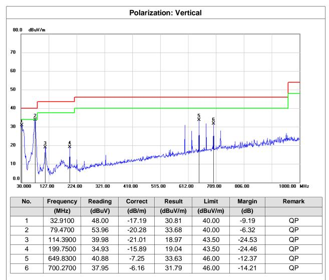
Result = Reading +Correct (Amplifier Factor + Cable Loss + Antenna Factor) Margin = Result - Limit
