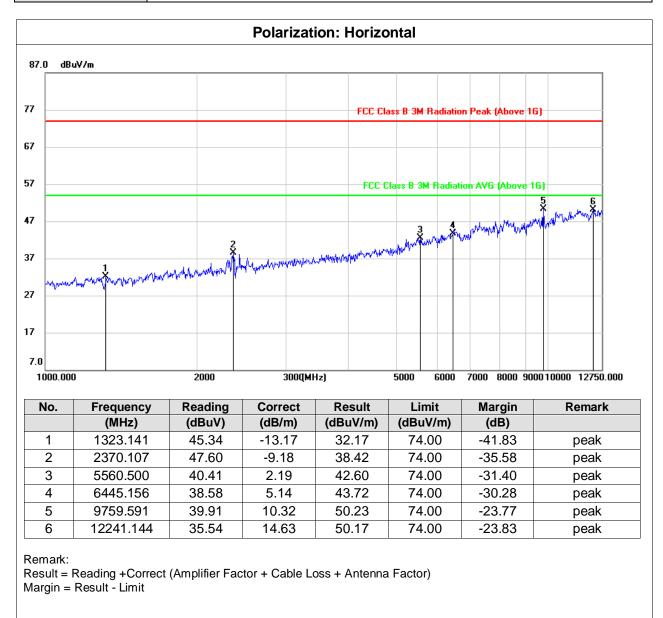
Note: All constructions have been tested, only the worst data of test construction 1 record in the report.
