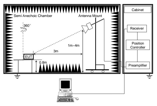
Note : For all radiated test, EUT in each of three orthogonal axis emissions had been tested, but only the worst case (X axis) data recorded in the report.
