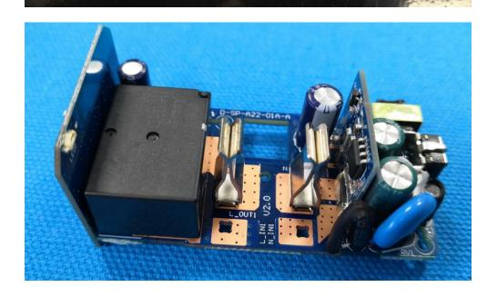
AZ9481 Relay , without power analyzer chip
