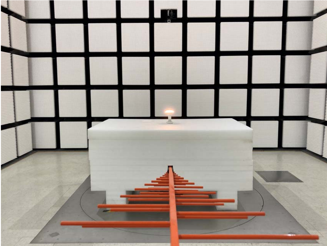
Radiated Emission Above 1GHz View
