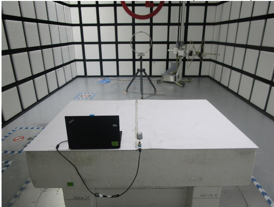
RADIATED RF MEASUREMENT SETUP (Below 30MHz)
