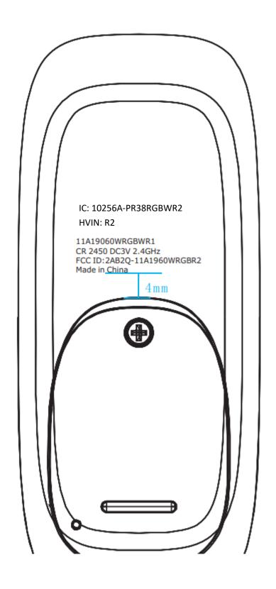
Note: the label is on the back of the device through silk-screen printing.
