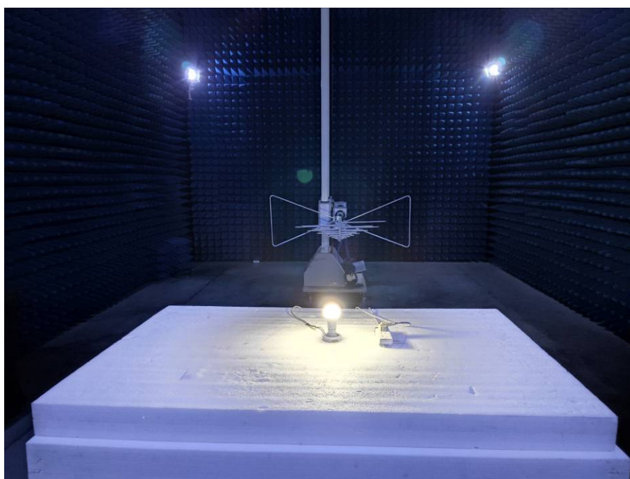
Photo of Radiated Emission Measurement (Below 1G)
