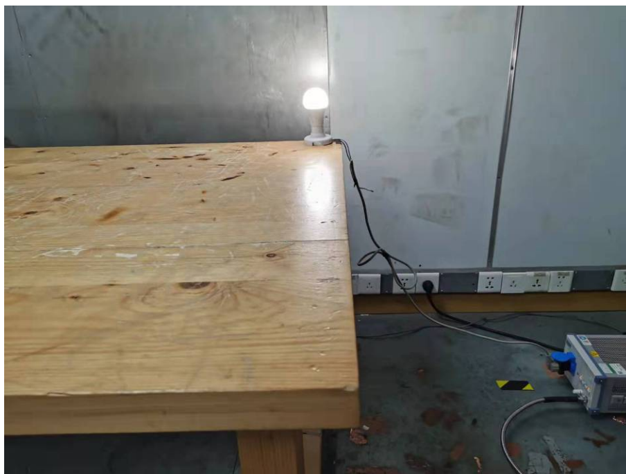
Photo of Conducted Emission Measurement
