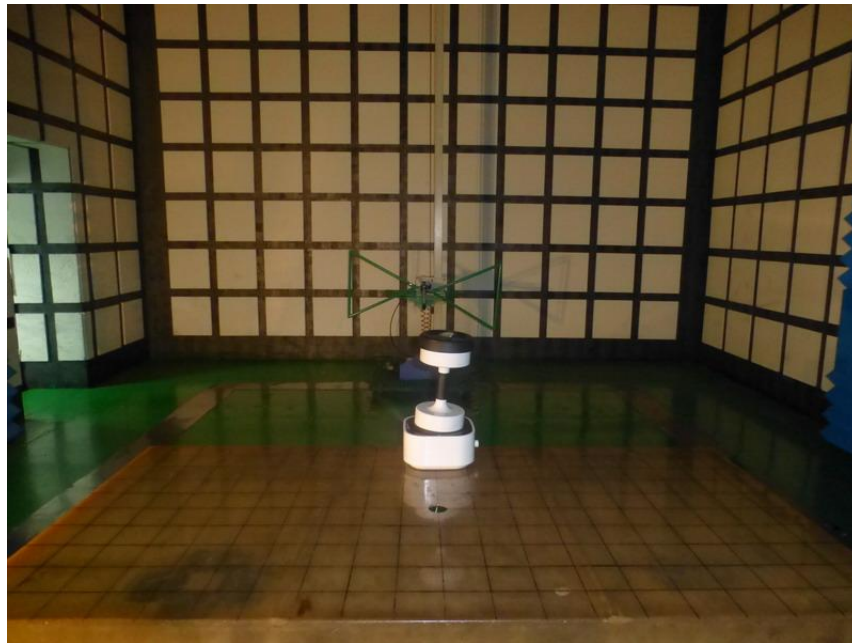
Photograph 3: Radiated Emission Test Configuration, (30-1000MHz) Front
