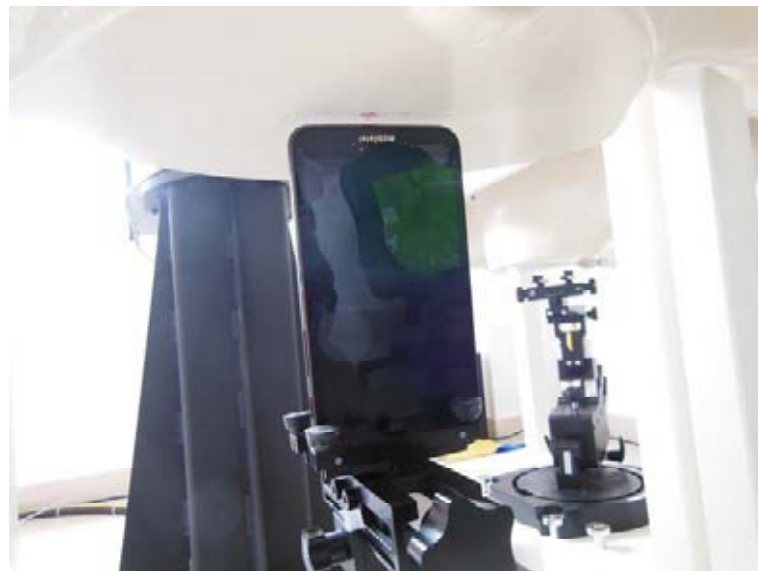
10mm Body-worn Top Side Setup Photo
