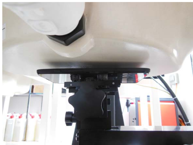
10mm Body-worn Rear Setup Photo
