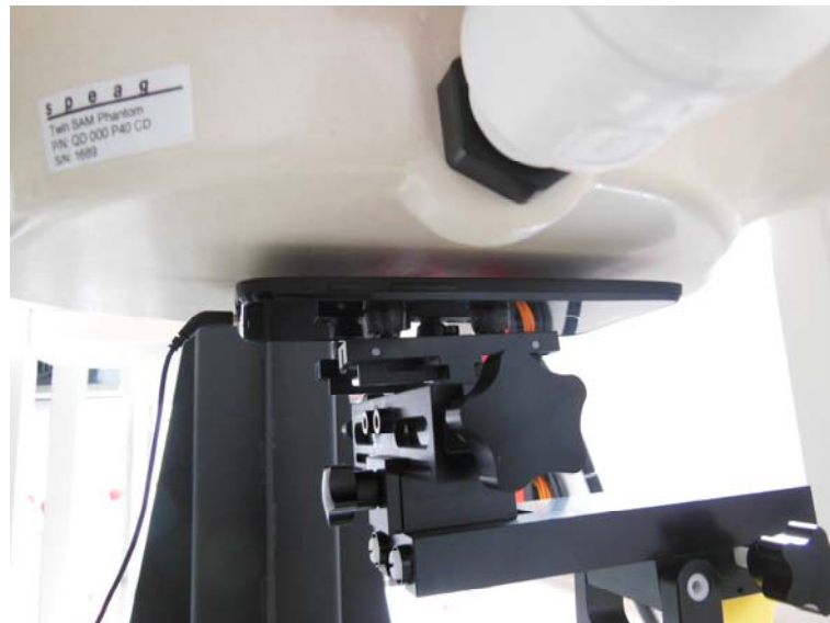
10mm Body-worn Rear (With Headset) Setup Photo
