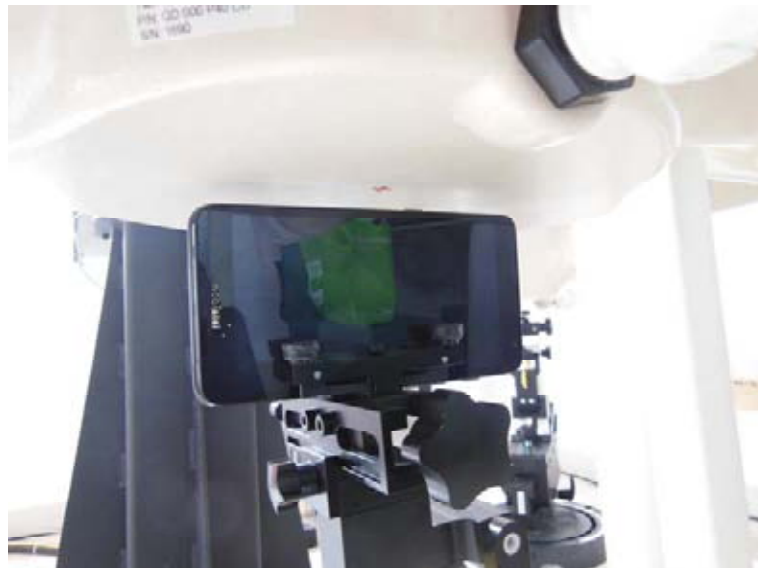
10mm Body-worn Right Side Setup Photo
