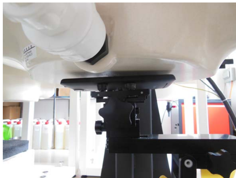
10mm Body-worn Front Side Setup Photo
