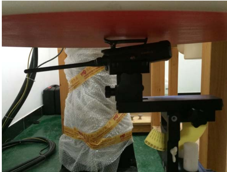
Body-worn, the front of the EUT towards ground with A1, B2, BC2 and C1 (The distance was 0mm)
