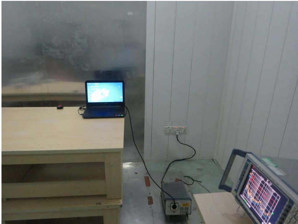
FCC RADIATED EMISSION TEST SETUP
