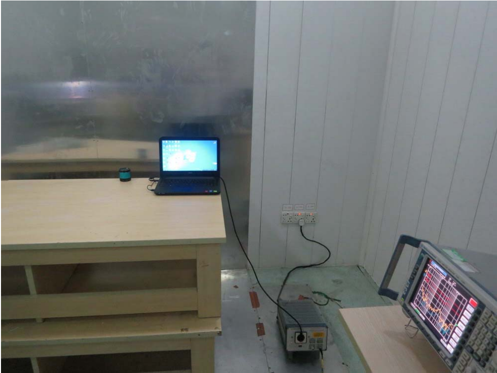
FCC RADIATED EMISSION TEST SETUP
