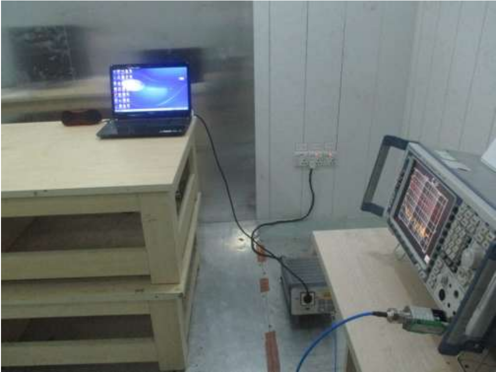
FCC RADIATED EMISSION TEST SETUP
