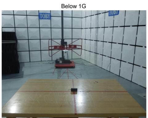
Radiated Spurious Emission Test Setup
