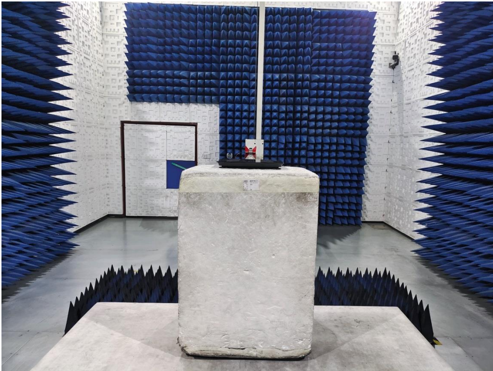
RADIATED EMISSION TEST SETUP ABOVE 1GHZ
