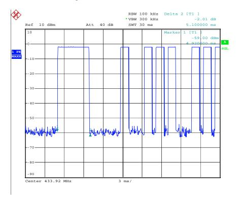
The graph shows the duration of 'on' signal. From marker 1 to marker 1, duration is 5.10ms.
