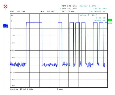
The graph shows the duration of 'on' signal. From marker 1 to marker 1, duration is 1.38ms.
