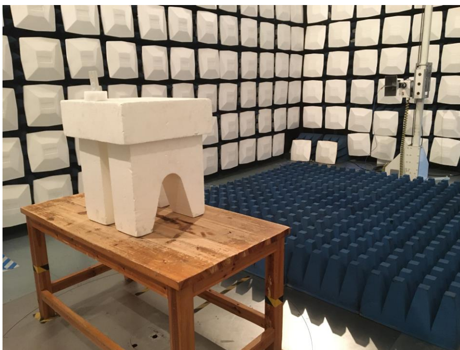
Test Setup For Radiated Emission (Above 1GHz)
