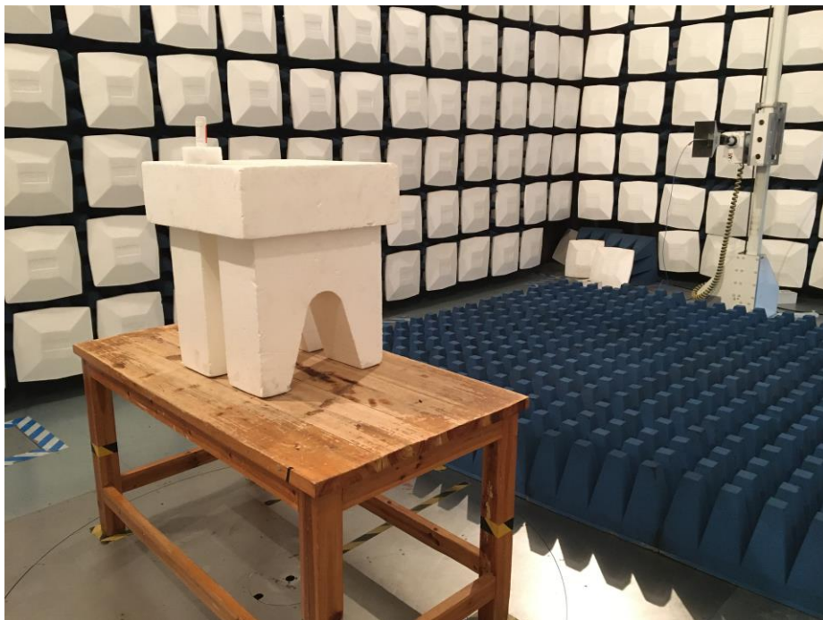
Test Setup For Radiated Emission (Above 1GHz)
