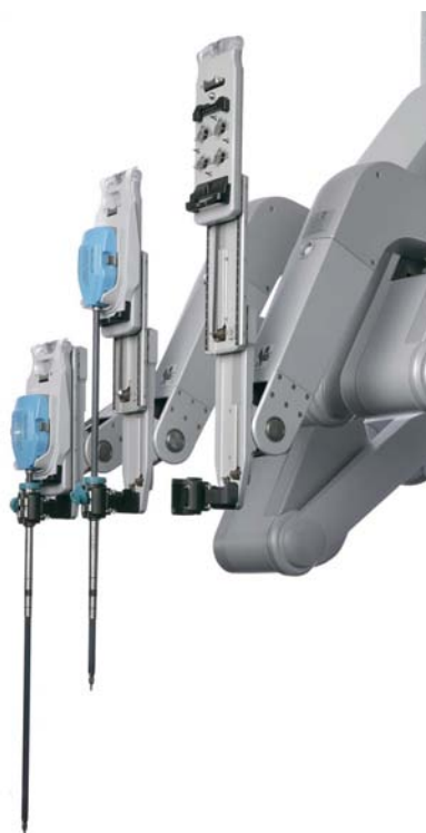
Figure 9.1 Instruments installed on the insertion axes
