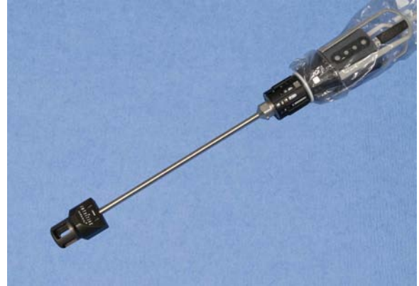
Figure 7.16 Alignment target and scope tip inserted, target centered on screen
