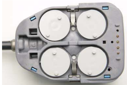
Figure 9.6 Discs located in the instrument housing
