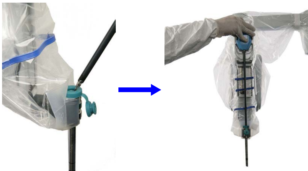
Figure 9.8 Inserting the instrument into the cannula and sterile adapter
