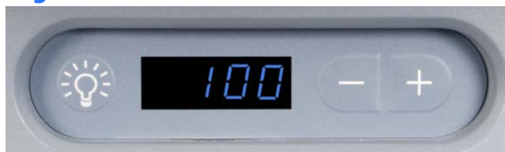
Figure 7.18 Illuminator controls and intensity display
