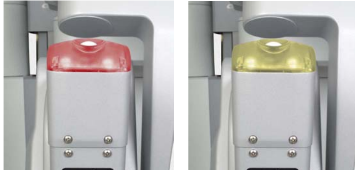
Figure A.2 Arm LEDs in fault states
