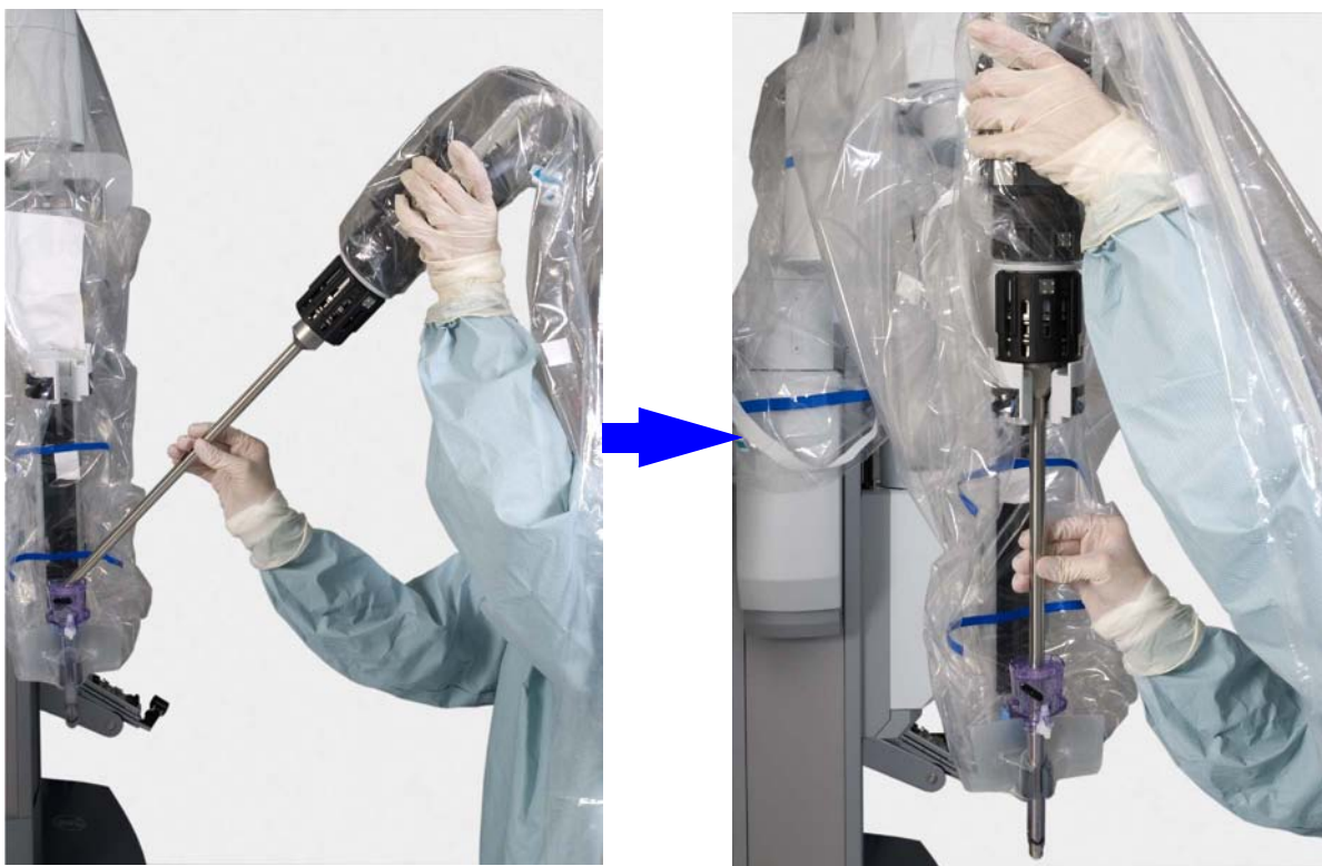
Figure 9.16 Installing the endoscope on the camera arm
