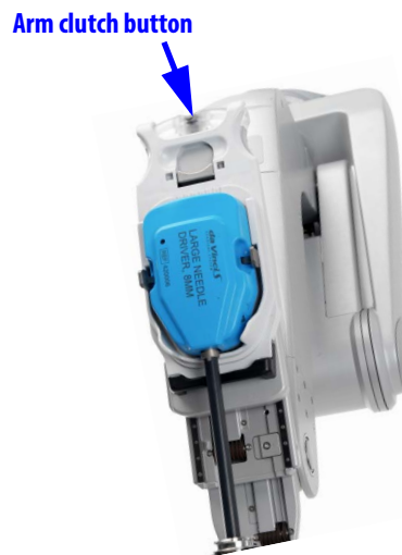
Figure 9.9 Using arm clutch to insert an instrument manually
