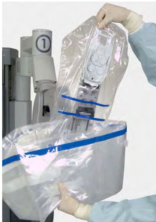
Figure 6.9 Lowering the drape over the insertion axis
