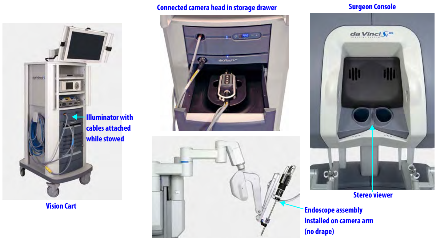
Figure 7.1 Vision system components
