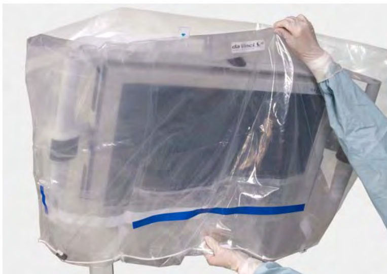
Figure 6.24 Lower the drape over the monitor
