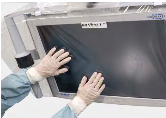
Figure 6.27 Smoothing the drape on the monitor
