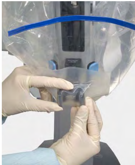
Figure 6.18 Seating the cannula mount molding
