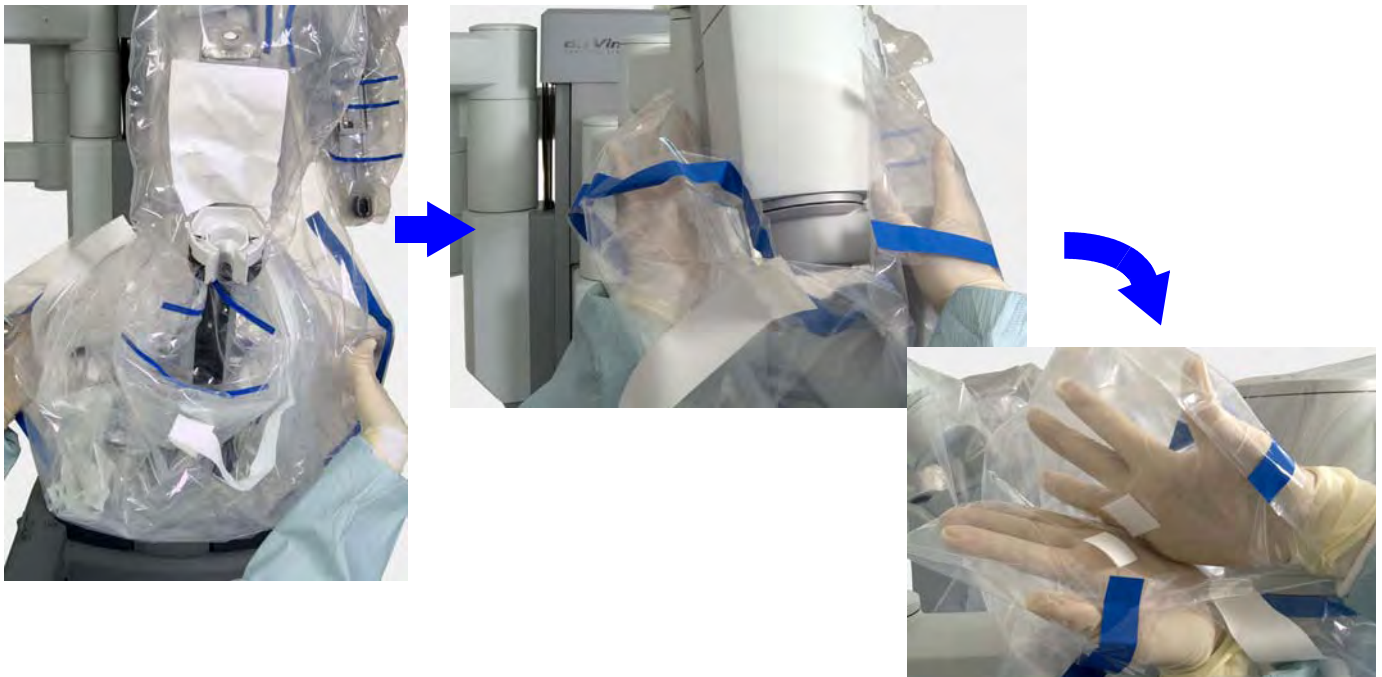
Figure 6.17 Extend drape to the center column and secure
