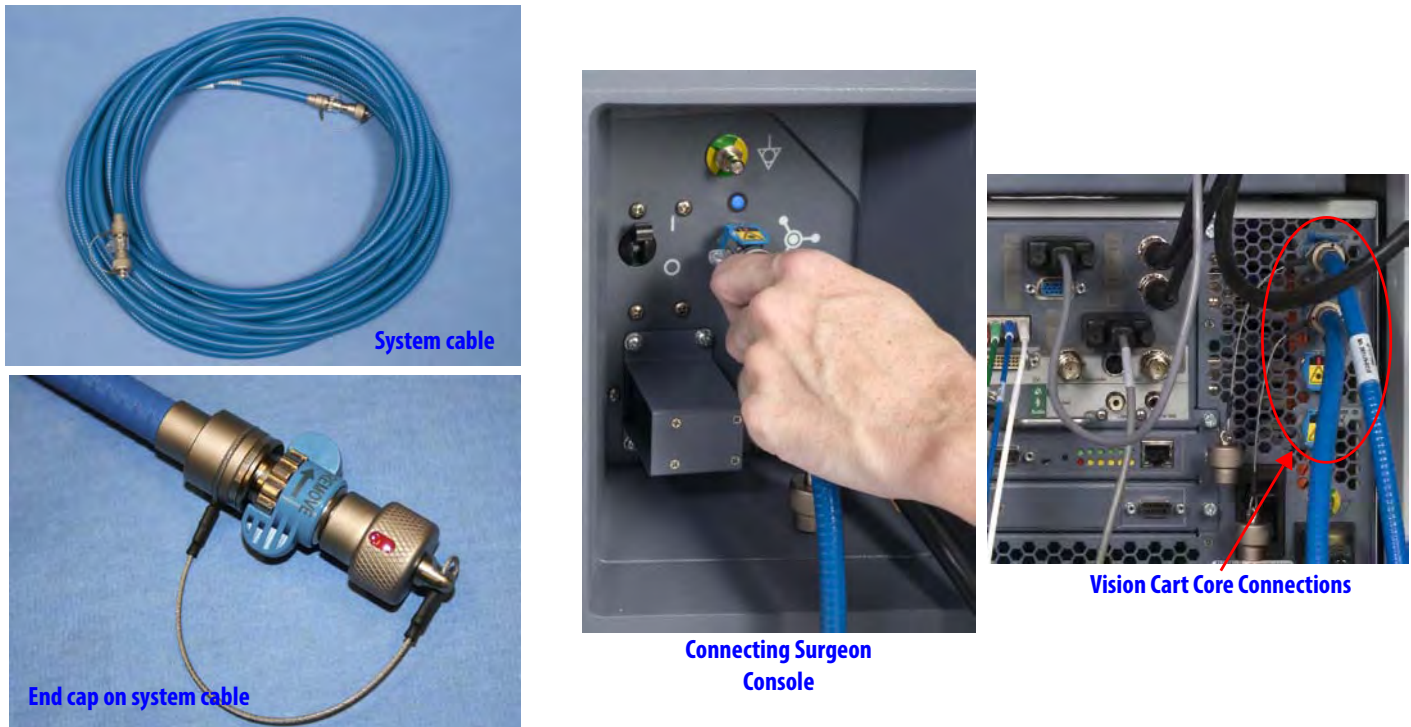
Figure 4.1 Sample system cable and connections
