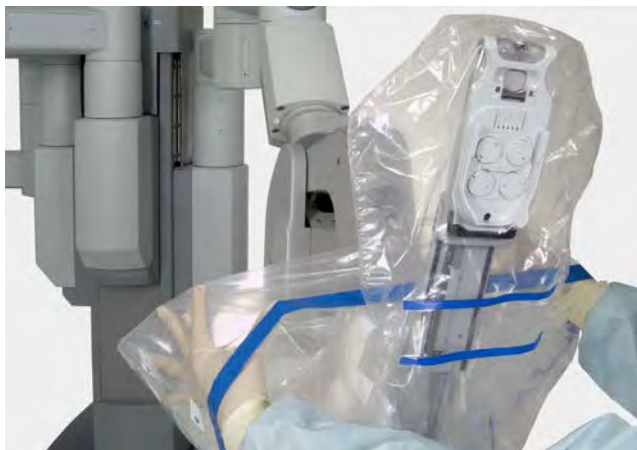
Figure 6.11 Stretching the drape along the arm
