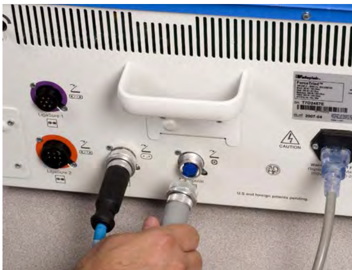
Figure 4.13 Auxiliary device connection (back of ESU)
