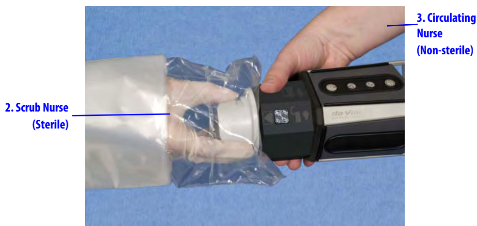
Figure 6.21 Attaching camera head to sterile adapter
