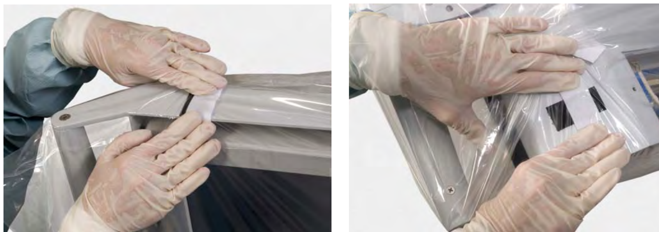
Figure 6.28 Secure Velcro straps on sides and rear
