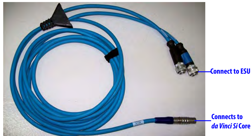
Figure 4.11 Representative Auxiliary Device Cable
