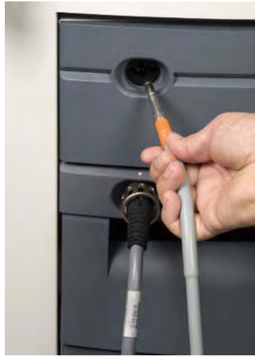
Figure 4.8 Connecting the light guide cable
