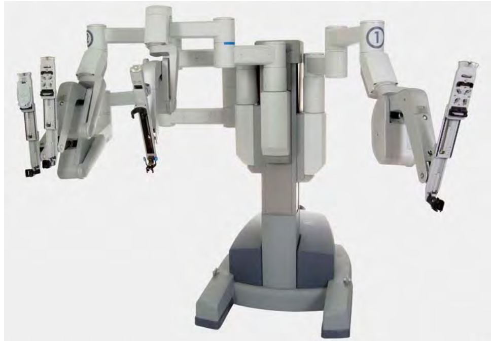
Figure 5.4 Instrument arms extended for draping
