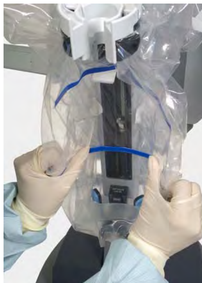
Figure 6.20 Bend the blue flex-strips around the insertion axis
