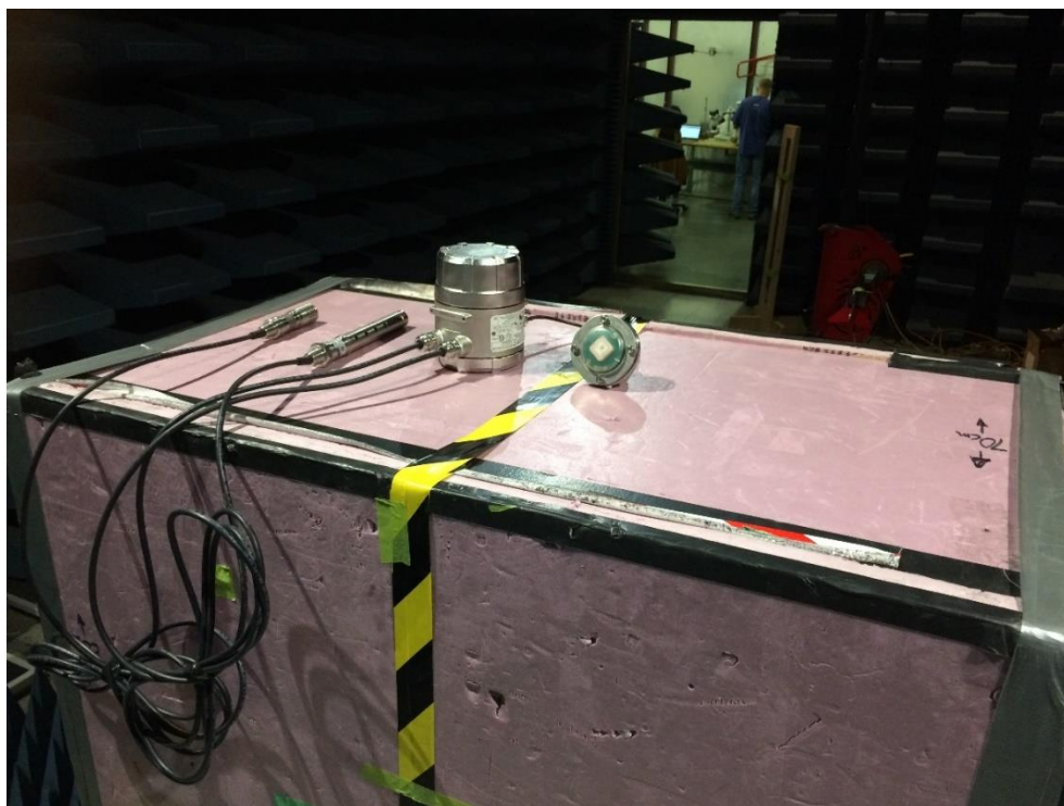
Test Setup, the EUT with RH circular antenna
