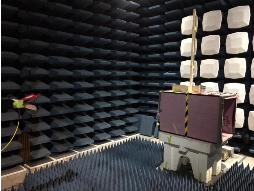
Radiated Emissions (frequency range: 1GHz ↔ 18GHz) Test Setup, the EUT with Omni-directional antenna
