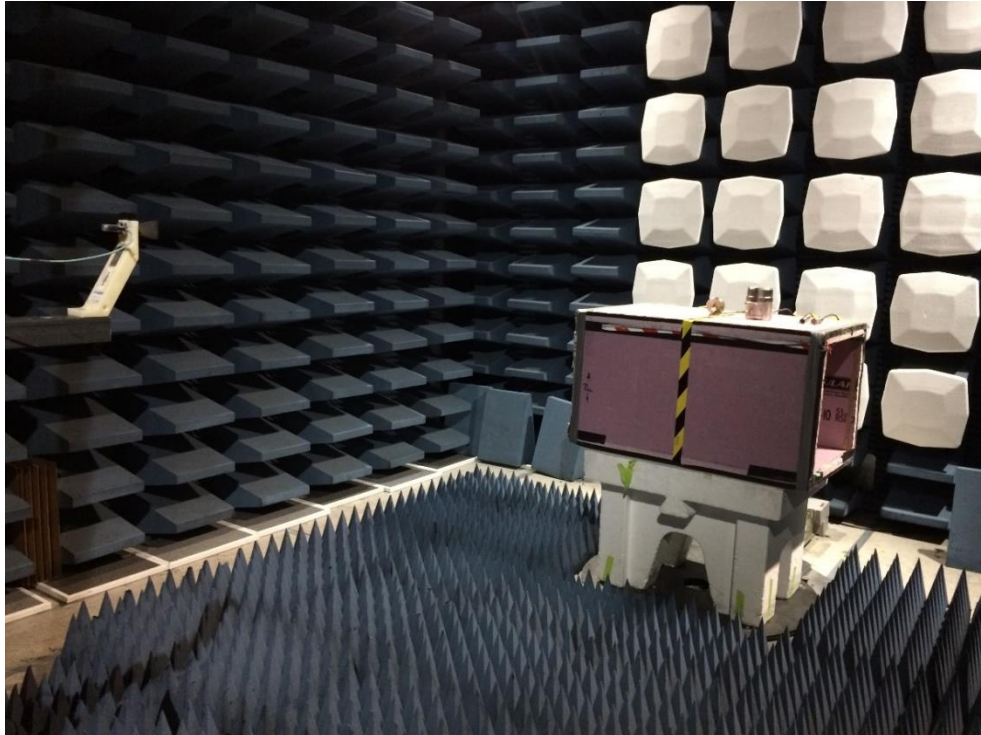
Radiated Emissions (frequency range: above 18GHz) Test Setup, the EUT with RH circular antenna
