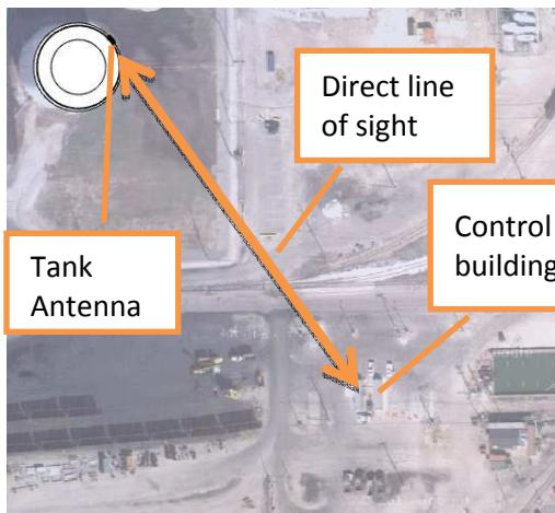
The Base-Station antennas can be located anywhere in the vicinity of the control building as it is far enough from the tank to not require a minimum antenna height.
