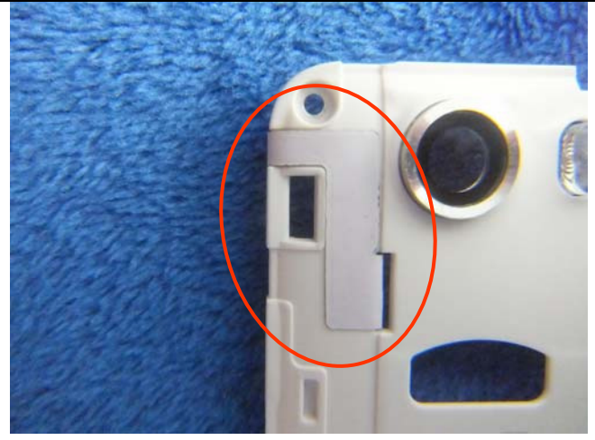
LTE Antenna View
