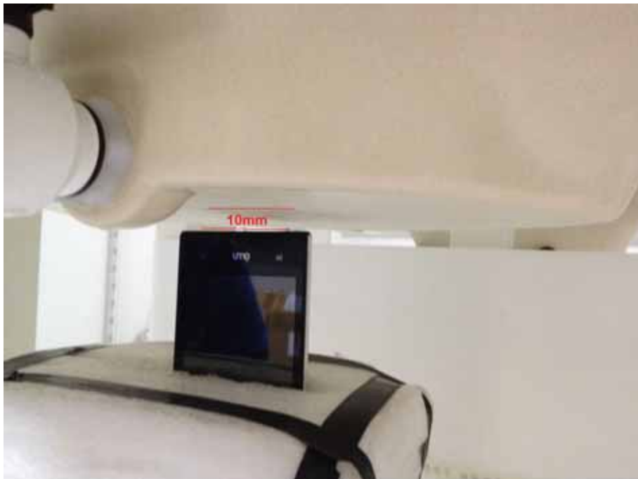
Body SAR Bottom 10mm for GSM/UMTS
