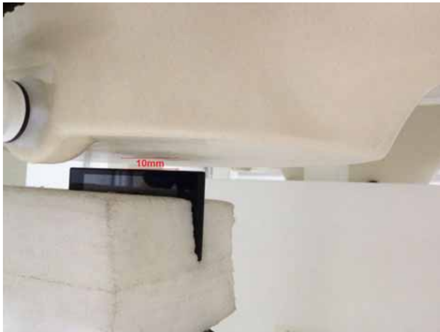
Body SAR Right Side 10mm for GSM/UMTS
