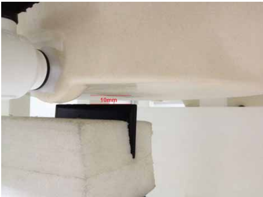
Body SAR Left Side 10mm for GSM/UMTS
