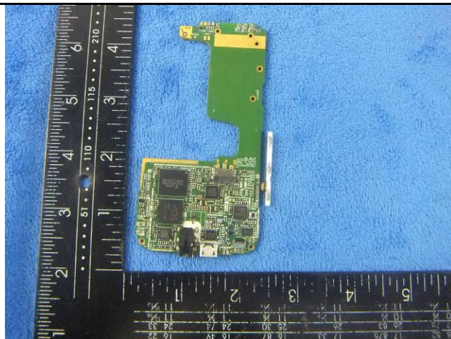
Mainboard without Shielding - Front View
