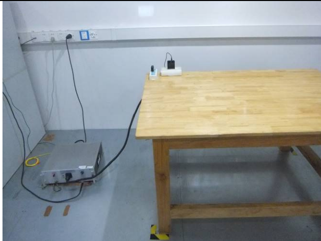
Conducted Emissions Test Setup Front View
