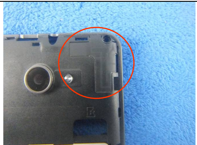
WIFI/BT/BLE/GPS - Antenna View
