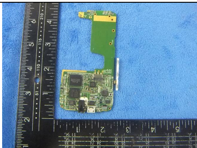
Mainboard without Shielding - Front View
