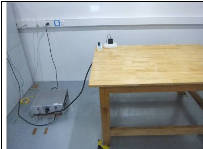
Conducted Emissions Test Setup Front View
