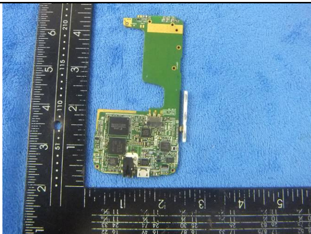
Mainboard without Shielding - Front View
