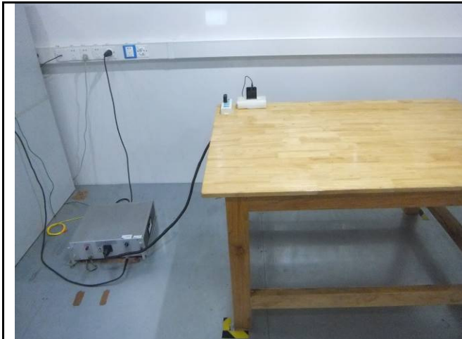
Conducted Emissions Test Setup Front View
