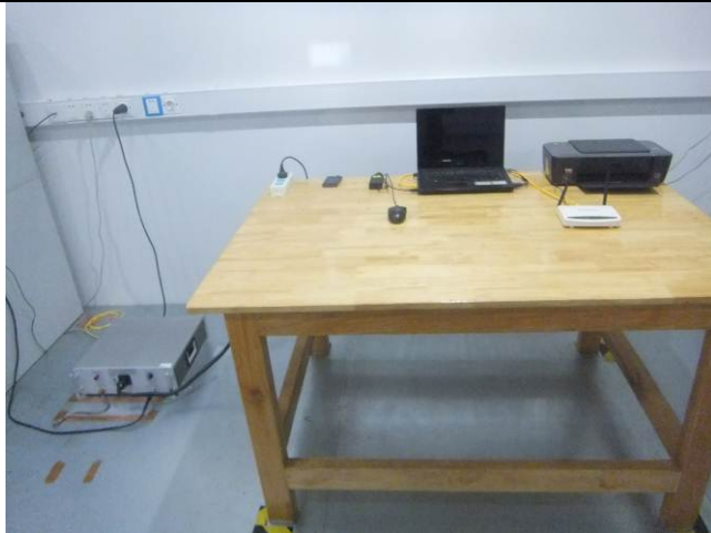
Conducted Emissions Test Setup – Front View
