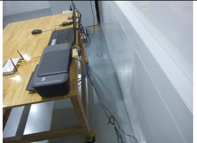
Conducted Emissions Test Setup – Side View
