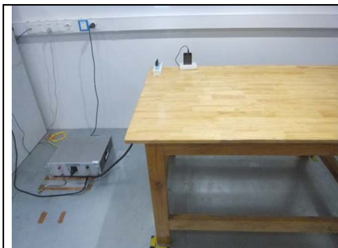
Conducted Emissions Test Setup Front View
