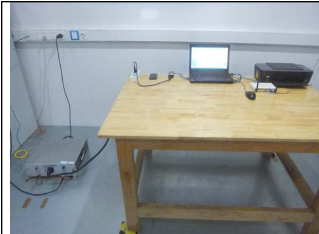
Conducted Emissions Test Setup – Front View
