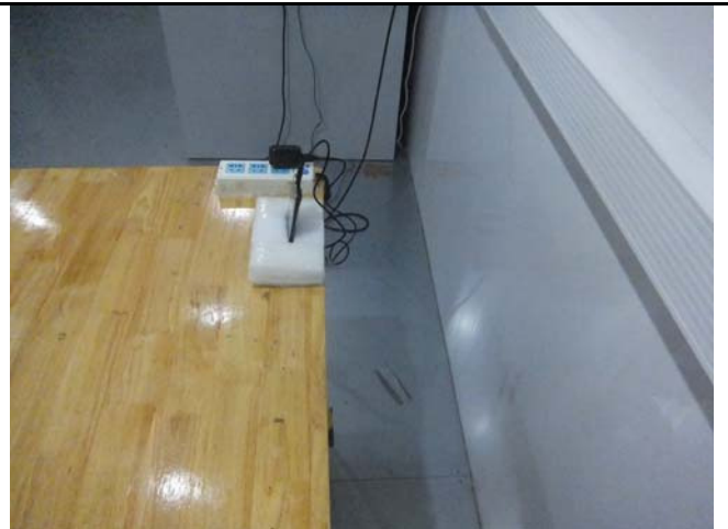
Conducted Emissions Test Setup Side View
