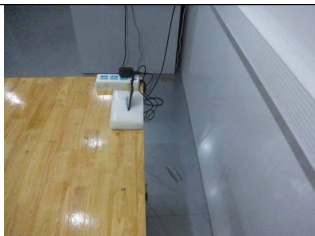
Conducted Emissions Test Setup Side View
