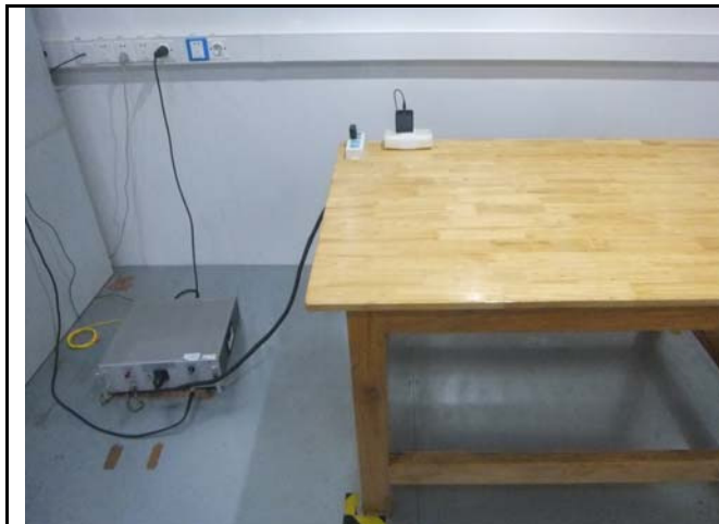
Conducted Emissions Test Setup Front View
