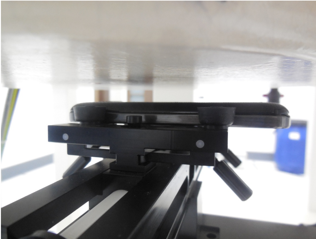
Band850, Band1900 and WIFI Test Setup Body Back with gap 10mm
